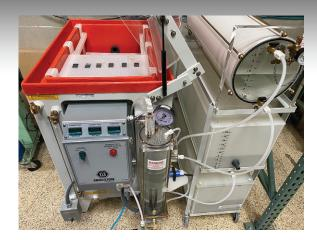
**STEP 4:** Setup environmental chamber for humidity and heat/cool cycle.
