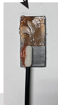
STEP 3: Using swab, wipe grease off half the coupon. Let sit on coupons for 24 hours.
