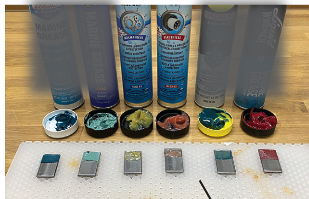
STEP 3: Using swab, wipe grease off half the coupon. Let sit on coupons for 24 hours.
