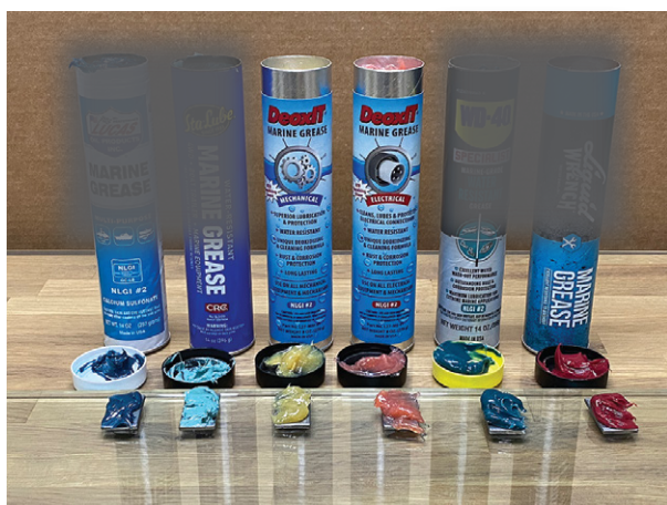
STEP 2: Treat/apply greases to entire coupon. Let sit on coupons for 24 hours.
